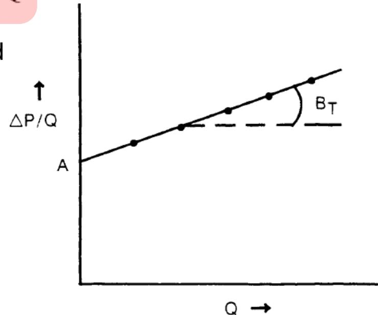
Fig. 7-40. Relationship between  $\Delta P$  and  $Q$  for the evaluation of parameters  $A$  and  $B_T$ .
