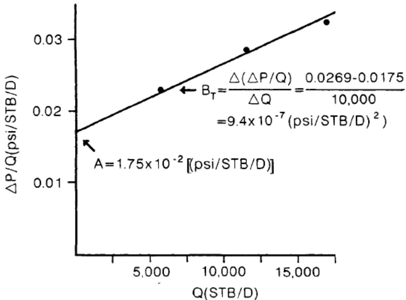
Fig. 7-41. Relationship between  $\Delta P/Q$  and  $Q$  obtained from well testing data in a fractured reservoir.
