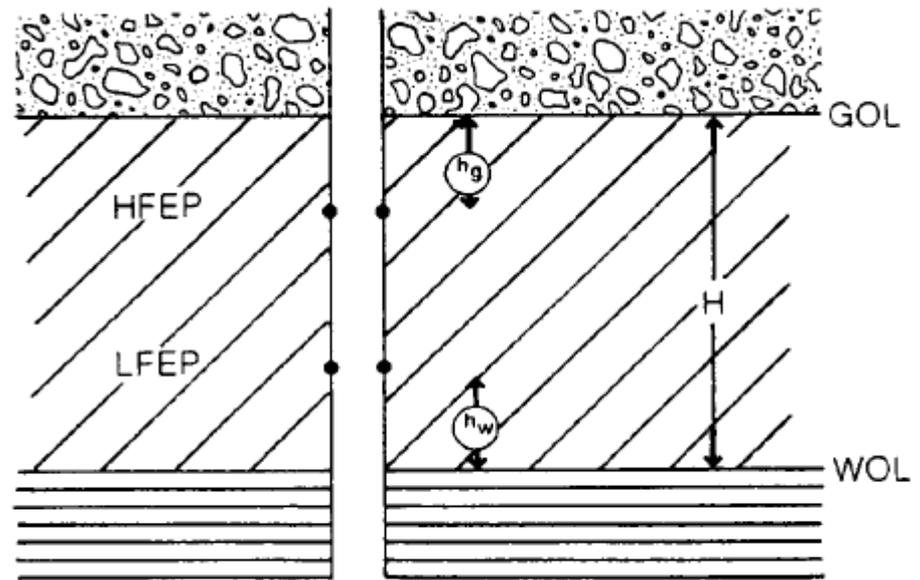
Fig. 7-42. Sketch of water-oil and gas-oil contacts vs. *LFEP* and *HFEP*.
