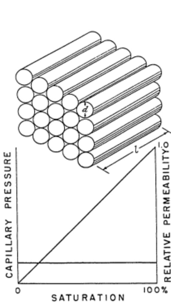
Fig. 31 - Hypothetical Capillary-pressure Curve for Bundle of Capillaries with Uniform Lengths and Uniform Diameters
