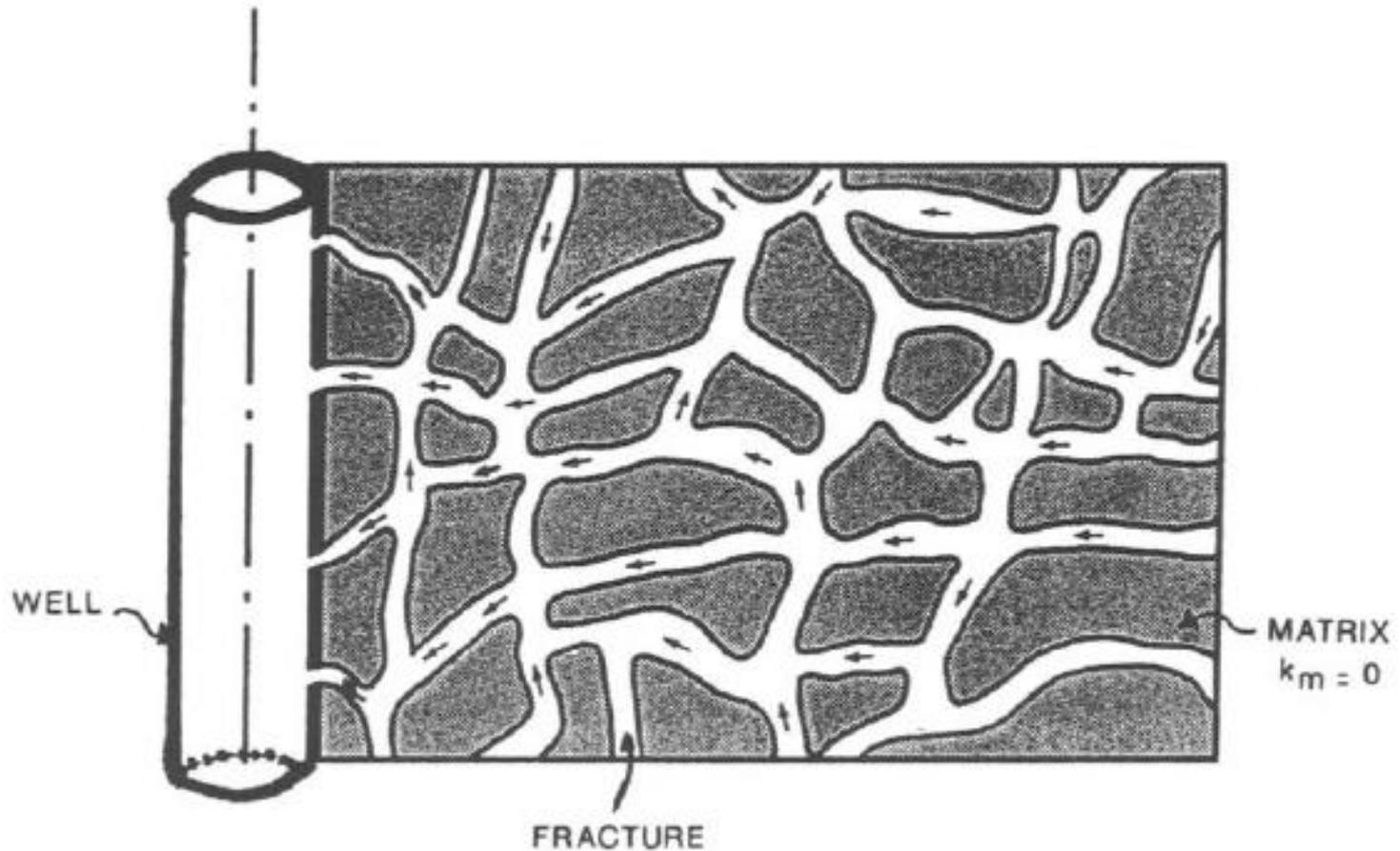
Fig. 7-38. Flow toward a well through fracture network.
