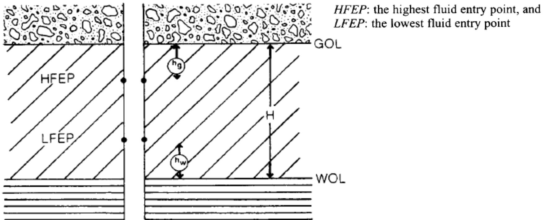
Fig. 7-42. Sketch of water-oil and gas-oil contacts vs. *LFEP* and *HFEP*.
