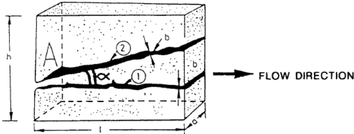
Matrix block containing two fractures. Fracture 1 ( $\alpha = 0$ ). Fracture 2 ( $\alpha > 0$ ).
