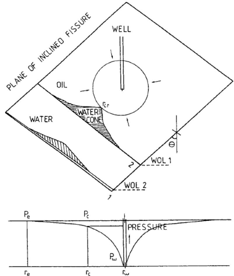
Fig. 7-43. Water coning, function of movable water-oil contact position.
