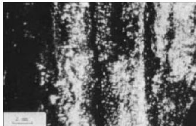
Figure 14-5. Thin section of a layered matrix deposit. The black layers are organic deposits, and the clear (white) layers are inorganic scales of mainly halite ( \text{NaCl} ).
