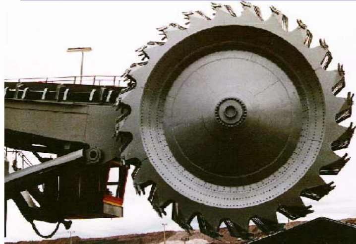
Bucketwheel with integrated buckets
