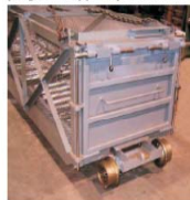
Materials Handling Car slung inside Counterweight
