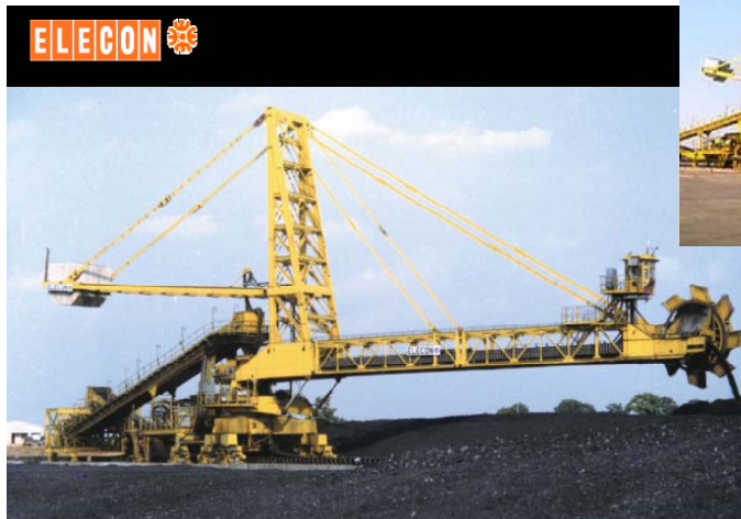
Reversible Type Bucket Wheel Stacker-cum-Reclaimer. Capacity 2,000 TPH of coal
