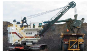
495 Electric Rope Shovel with Rope Crowd 100 tonnes (110 ton) nominal payload (Available dipper payloads to 120 tons (109 tonnes)) Dipper capacities: 26.8 to 61.2 m 3 (35 to 80 yd 3 )
