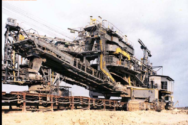
Crawler-mounted Tripper, weighing 500 tones in operation at Neyveli Lignite Corporation's open cast mine handling overburden at 11,000 tones/hr.
