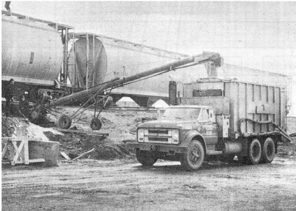
FIGURE 4.23: AN/FO TRUCK BEING LOADED DIRECTLY FROM AN AMMONIUM NITRATE RAIL CAR.
