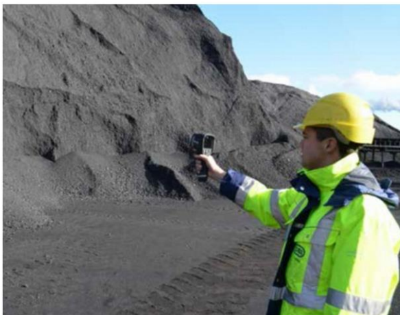
OBA combines the use of a temperature probe – the traditional way of measuring temperatures– and a FLIR E6 handheld thermal imaging camera.
