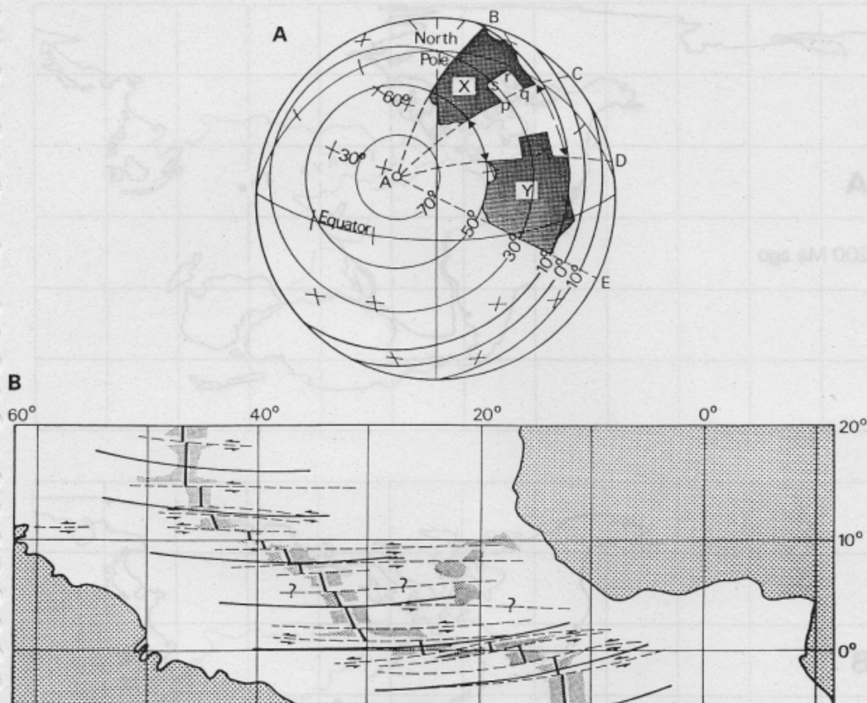
Fig. 2.15 The geometry of plate motion: (A) the movement of two segments of the Earth's surface with respect to a common pole of rotation; (B) the alignment of transform faults (dashed lines) in the equatorial Atlantic compared with small circles (solid lines) concentric about a pole located at 58^{\circ}\text{N} , 36^{\circ}\text{W} . (After E. R. Oxburgh (1971) in: I. G. Gass, P. J. Smith and R. C. L. Wilson (eds) Understanding the Earth . Open University Press, Milton Keynes, Figs. 19.2 and 19.3, p. 266.)
