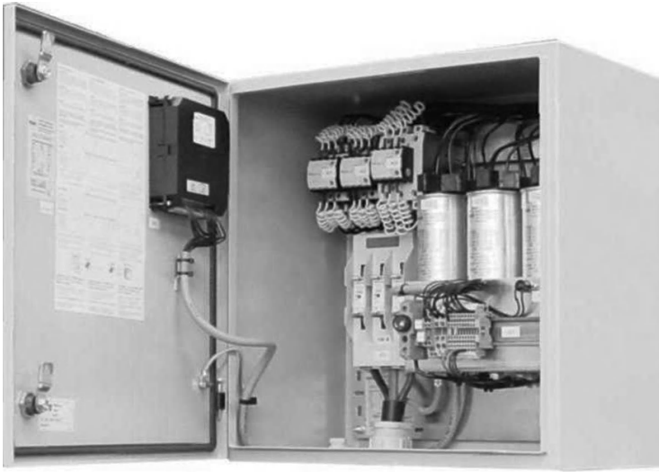
Figure 11.16b Compensation bank for wall mounting of 52.5 kvar; 400 V, 50 Hz; switching in seven steps \times 7.5 kvar. Reproduced by permission of Frako Kondensatoren und Anlagenbau GmbH, Germany.
