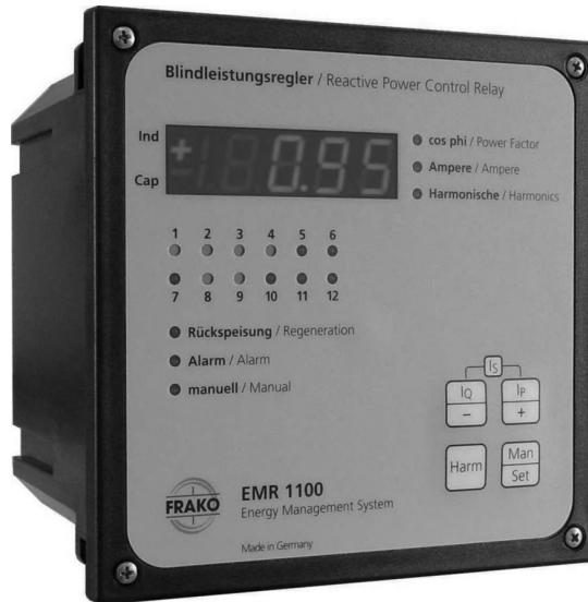
Figure 11.5b Reactive power control relay: 400 V/230 V, 50 Hz; 12 control outputs; suitable for four-quadrant-operation. Reproduced by permission of Frako Kondensatoren und Anlagenbau GmbH, Germany.
