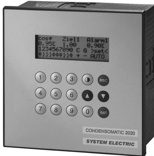
Figure 11.5c Reactive power controller CONDENSOMATIC 2020: up to 700 V measuring voltage; 50/60 Hz; x A/5 A/1 A; dynamic type:13 ms for switch command; 10 control outputs; suitable for four-quadrant operation. Reproduced by permission of System Electric GmbH, Germany.
