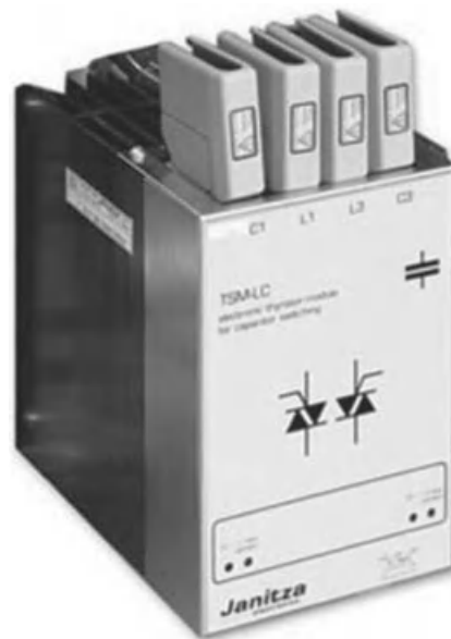
Figure 14.5b Static contactor (thyristor module fitted with two thyristors and two anti-parallel diodes) for contactless switching of three-phase power capacitors up to 100 kvar, 400 V, type TSM-LC. Reproduced by permission of Janitza Electronics GmbH, Germany.
