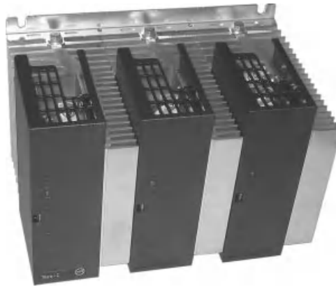
Figure 14.6b Static contactor (thyristor module fitted with three thyristors and three anti-parallel diodes) suitable for the control of capacitors with rated voltage higher than 500 V. Reproduced by permission of Maschinenfabrik Reinhausen GmbH, Germany.
