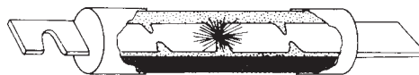
(b) The link melts and an arc is established under sustained overload current
