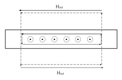
In taking the line integral in Ampere's law, the two vertical path segments will cancel each other. Ampere's circuital law for the interior loop becomes
