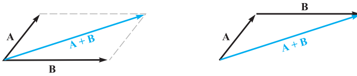
Figure 1.1 Two vectors may be added graphically either by drawing both vectors from a common origin and completing the parallelogram or by beginning the second vector from the head of the first and completing the triangle; either method is easily extended to three or more vectors.
