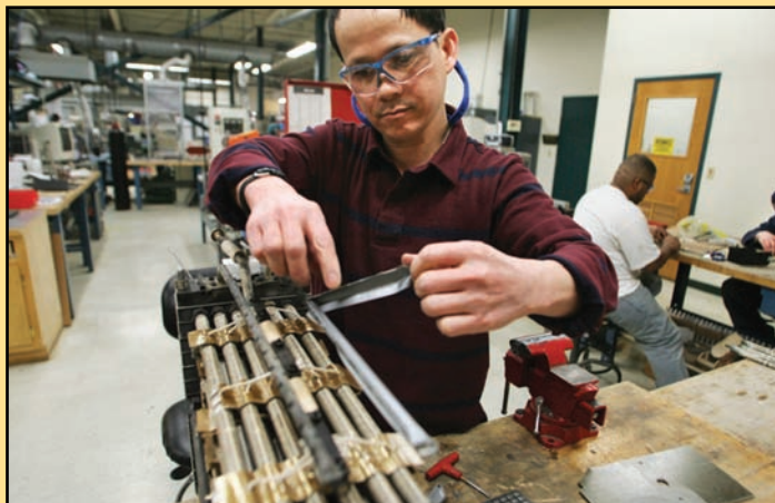
A worker in a Massachusetts plant assembles part of a fuel cell stack.
