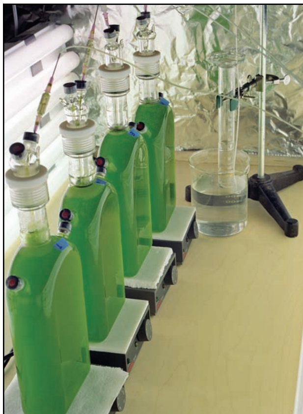
A system for producing hydrogen from algae.
