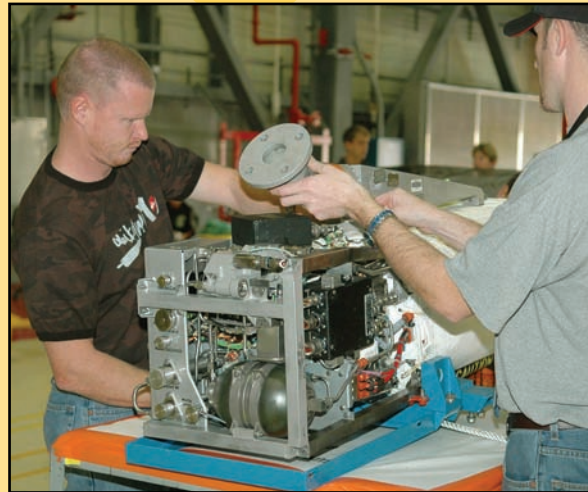
Workers take apart a fuel cell that has been removed from the space shuttle.
