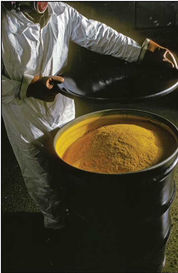
A technician with a barrel of yellowcake, which has been refined so that it is mostly uranium.
