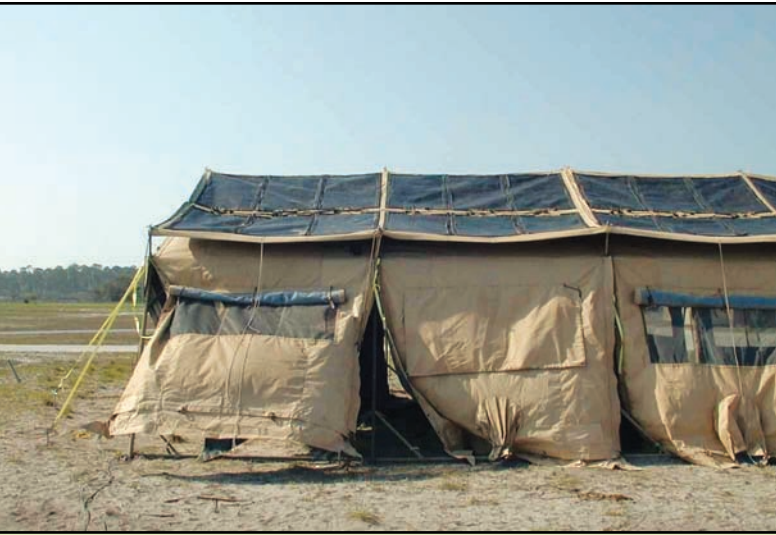
Some U.S. Army tents have thin-film solar cells. They provide power for such things as laptop computers and phones.
