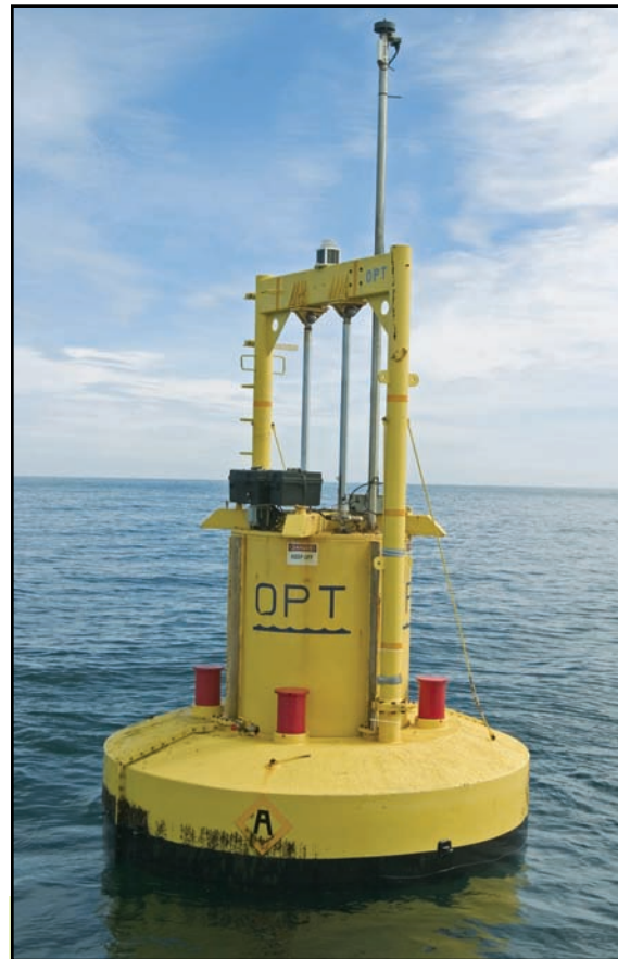
The PowerBuoy® system developed by Ocean Power Technologies, Inc., captures the natural energy in ocean waves.
