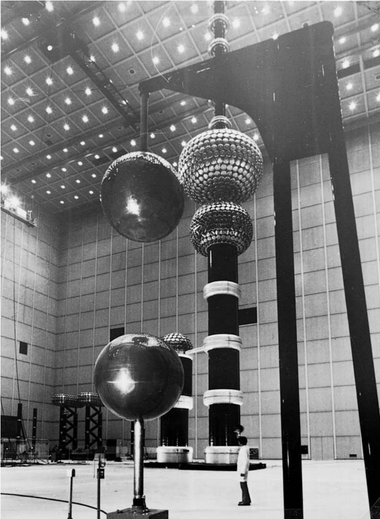
Figure 2.16 (a) Cascaded testing transformers with insulating shell construction (courtesy IREQ, Canada)
