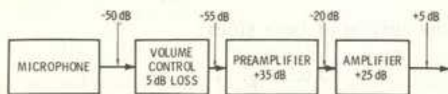
Figure 9-4. Block diagram of an amplifier, showing dB losses and gains.
