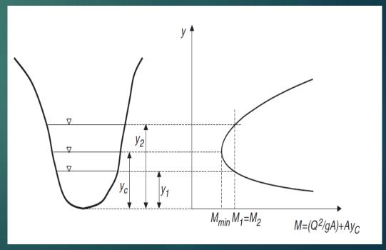
• These depths, marked as  $y_1$  (supercritical) and  $y_2$  (subcritical) in the figure, are called the conjugate depths (Henderson 1966).
