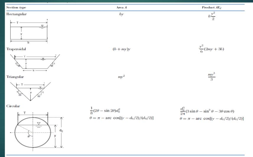
$Y_{\rm C}$  = vertical distance from the free surface to centroid of flow section (see Chapter 1).
