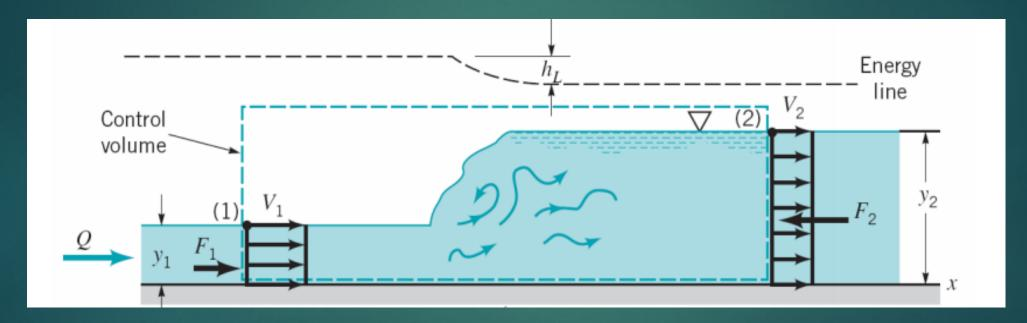
Conjugate depths refer to the depth (y<sub>1</sub>) upstream and the depth (y<sub>2</sub>) downstream of the hydraulic jump.
