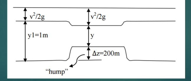
Q2-2. A rectangular channel b= 2.0 m, Q= 2 m3/s, the depth of uniform flow before the hump is 0.8 m. What should be the height of the hump ( $\Delta z$ ) to have critical flow over it (no head loss).
