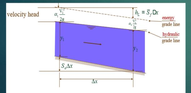
Bottom slope  $(S_o)$  not necessarily equal to EGL slope  $(S_f)$
