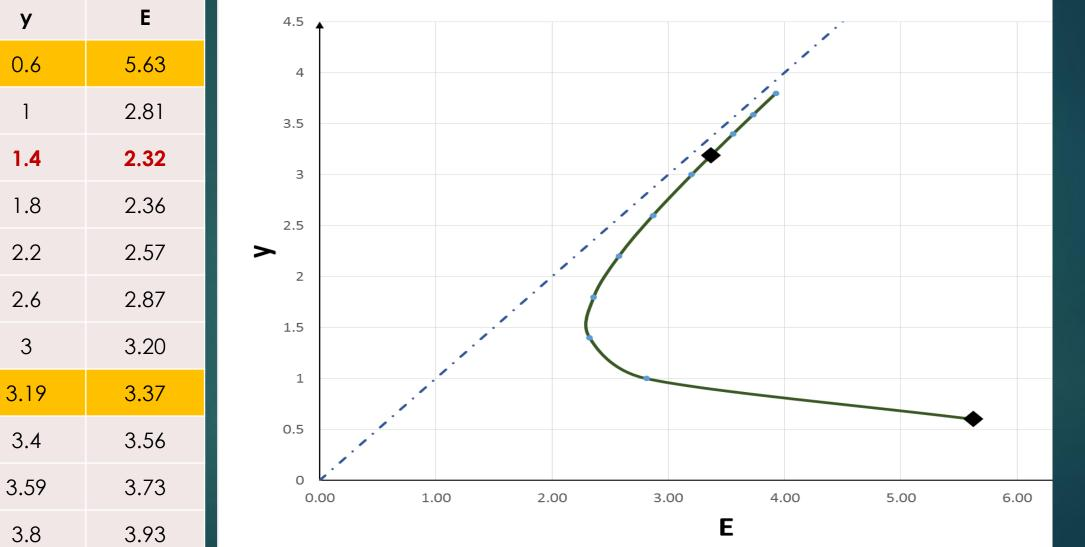
Q2-1. A rectangular channel b= 1.5m, Q= 900L/s, the depth of flow before the hump is 1m and  $\Delta z=200mm$ , compute the depth of flow above the hump.
