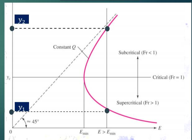
The specific energy diagram reveals that the flow needs the minimum specific energy, Emin, to pass a channel section at critical depth.
