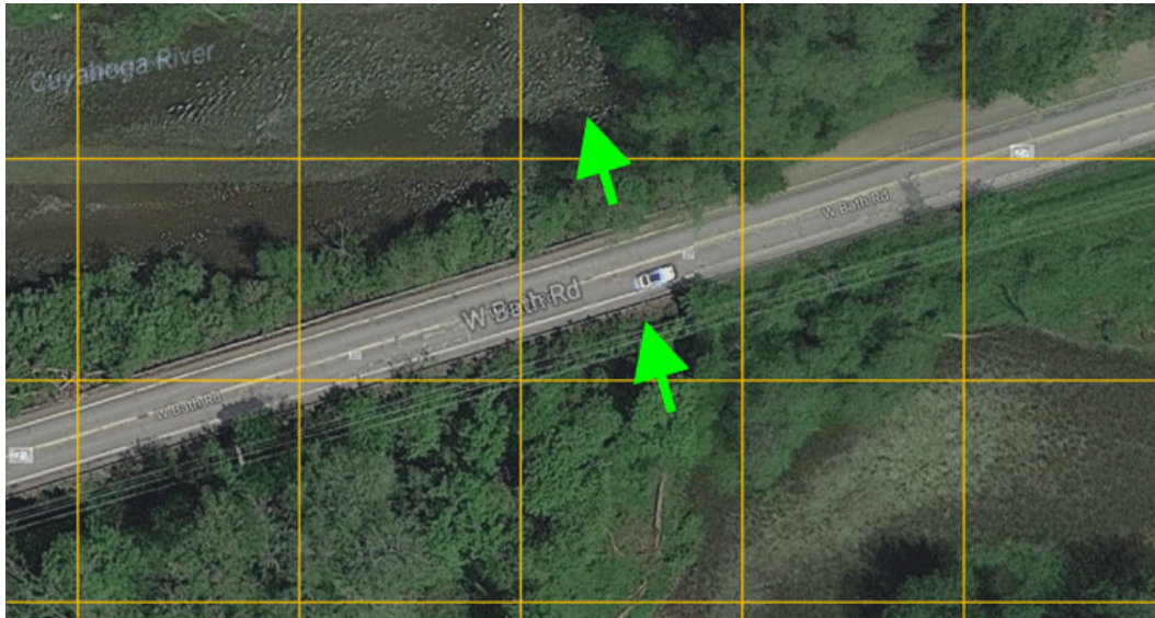
Example of 2D cell straddling element, causing flow to leak through the roadway crossing
