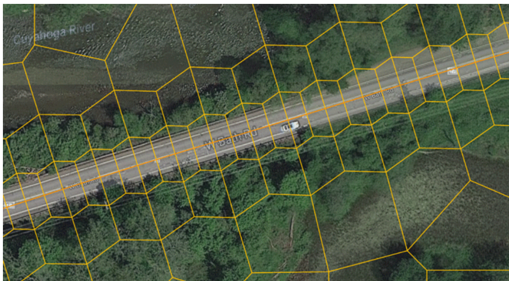
By aligning the cell faces with the structure, the leaking of flow is eliminated
