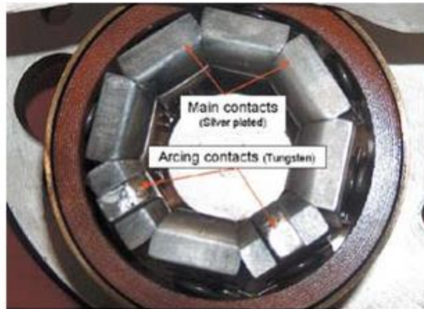
Tulip contact in oil circuit breaker
