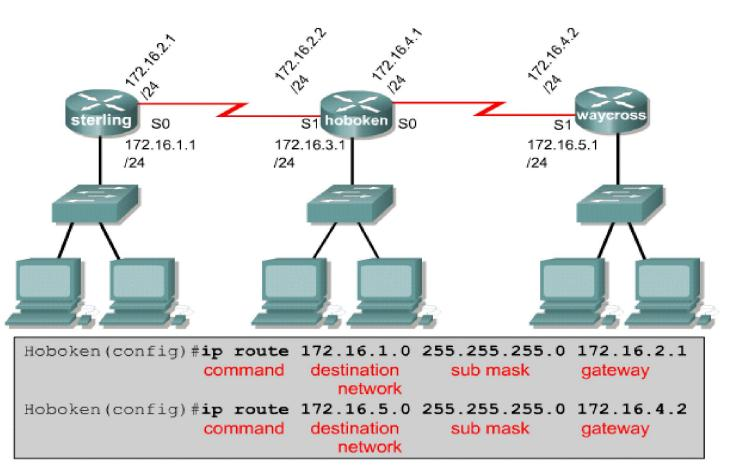
If the router cannot reach the outgoing interface that is being used in the route, the route will not be installed in the routing table.
