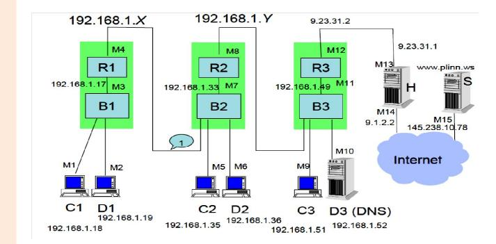
3. Instead of manual configuration as in question 2, routers R1 R2 and R3 use now RIP. After RIP has converged, what are the routing tables at each router? Give only the entries for destination prefixes that are not on-link with this router.
