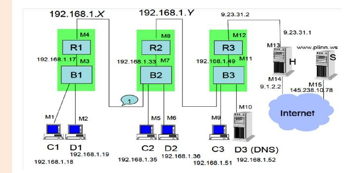
2. We assume that R1, R2 and R3 are manually configured, i.e. they do not run any routing protocol. Put in the table below the routing table entries that needs to be written in these three routers (to use static route i.e in R2). Give only the entries for destination prefixes that are not on-link with this router.
