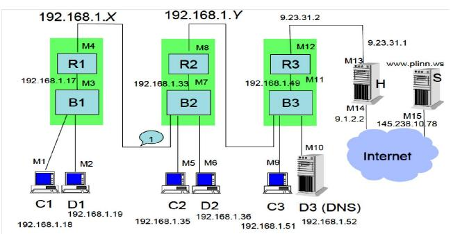
1. Give a possible value for the X in the IP address of the interface M4 of router R1 (i.e. give a possible value for the address marked 192.168.1.X on the figure). Justify your answer. Same question for the Y in the IP address of the interface M8 of router R2
