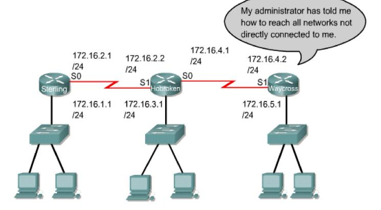
Waycross(config) **#ip route 0.0.0.0 0.0.0.0 S1** This command points to all non-directly-connected networks
