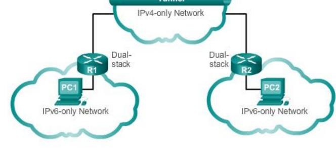
**Tunnelling**: A method of transporting an IPv6 packet over an IPv4 network. The IPv6 packet is encapsulated inside an IPv4 packet.
